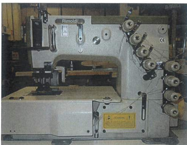
64R-41 MULTINEEDLE CHAINSTITCH MACHINE PREPARED TO ATTACH THE READY MADE BELT ON CLASSIC TROUSERS
