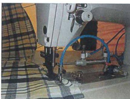
CF 3111 COMPLETE UNIT FOR SHIRT BOTTOM HEMMING OPERATION
