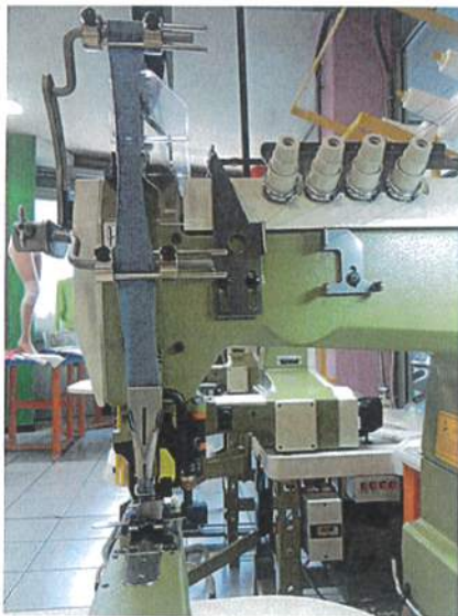
F17-34-1CD-13/358-RA LITTLE ARM OVERLOCK M/C FOR ELASTIC APPLICATION ON UNDERWEAR WITH ELECTRONIC CONTROL OF THE INSERTION-CUT-INSERTION OF THE ELASTIC AND ITS TENSIONING RATIO
