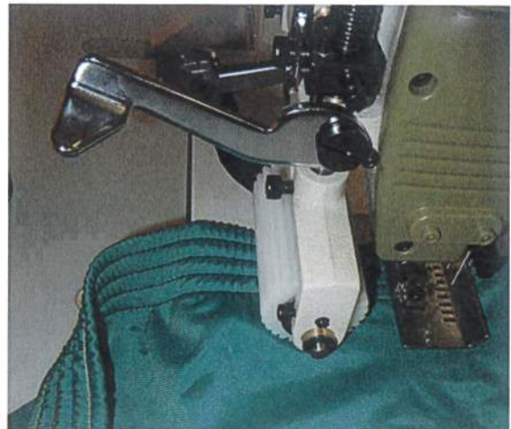
F84-38-2CA-01/164-15 APPLICATION OF A KNITTED STRIP ON SHOULDERS AND BACK OF NECK OF THE T-SHIRT
