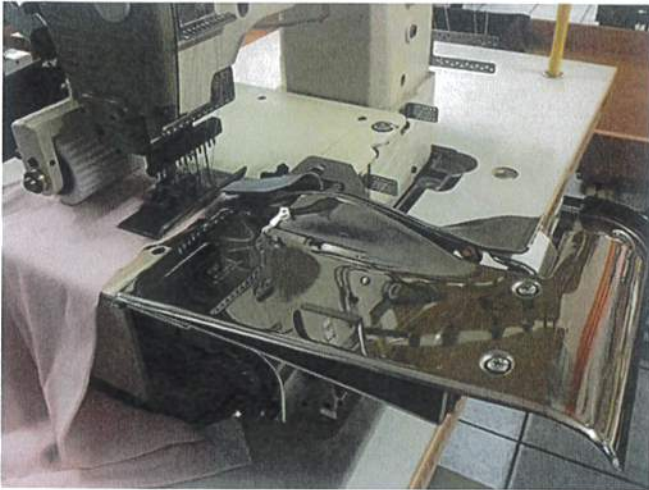
64R-11-0ML-01 ELASTIC APPLICATION ON BOXER
