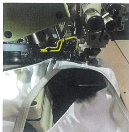
F17-34-1CD-13/358-RA LITTLE ARM OVERLOCK M/C FOR ELASTIC APPLICATION ON UNDERWEAR WITH ELECTRONIC CONTROL OF THE INSERTION-CUT-INSERTION OF THE ELASTIC AND ITS TENSIONING RATIO
