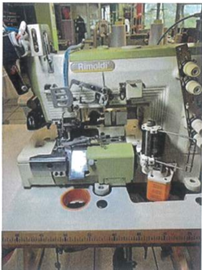
CF 3111 COMPLETE UNIT FOR SHIRT BOTTOM HEMMING OPERATION
