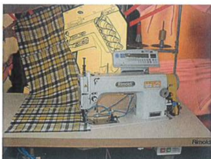
CF 3111 COMPLETE UNIT FOR SHIRT BOTTOM HEMMING OPERATION
