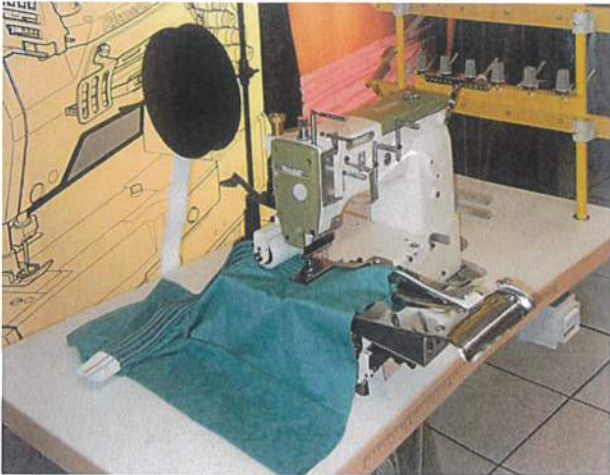
F84-38-2CA-01/164-15 APPLICATION OF A KNITTED STRIP ON SHOULDERS AND BACK OF NECK OF THE T-SHIRT
