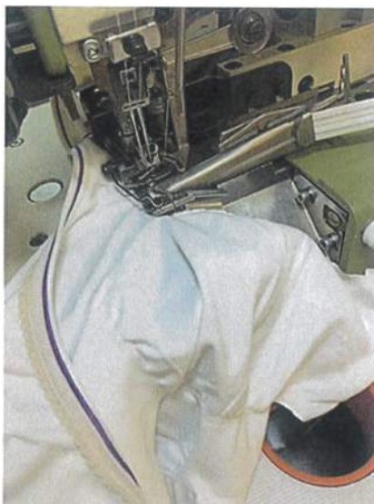
CF 3111 COMPLETE UNIT FOR SHIRT BOTTOM HEMMING OPERATION
