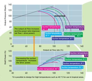
\*If the output flow rate exceeds the maximum capacity, motor overload protection function shall prevent intake of air.
