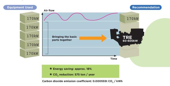
**Optimization**, the case where a large and powerful compressor is used with a large amount of air flow fluctuation:
