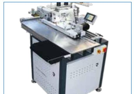
D-PH 510-IX and D-PH 610-IX are an Automatic Pocket Hemming units for jeans and similar sportswear/sportswear. The machine is equipped with a three needle **Kansai** chain stitch sewing head or alternatively a two needle **Brother** lock stitch sewing head. The machine performs the hemming on different fabric types (from heavy to stretch denim) through simple settings without a change of apparatus or parts. A single adjustable folder allows to single and double hem and change height
