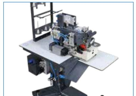
The machine D-WB 540-IX is designed for sewing waistbands of medium heavy to heavy material such as jeans, working pants, Sport pants and Skirts.
