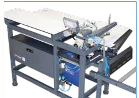
Automatic serging of denim trousers. The sewing unit D-SS 430-IX with Pegasus EXT 5214 offers excellent solutions for the rational serging of front and hind denim trousers parts. This automat has especially strengthened feeding and puller mechanisms as well as heavy duty stacker for denim fabric weight.
