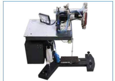
D-FA 420-M is a 3 needle, chain stitch Feed of the Arm automat specially designed for lap felling and/or double-lap seaming like yoke sewing, back seat, in-seam and side-seam operations for jeans, casual trousers in general, working clothes, denim jackets, etc.
