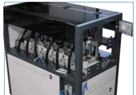
The Automat is used for automatic book-making of up to 8 different washing-care labels from Continuous Rolls of Labels. The automat cuts, optionally folds, collects & puts together 4 to 8 different sizes and lengths of care labels then carries them to the Bartack Sewing head. LB 631 - IX version is equipped with Ultrasonic Cutting system that can cut all various types of label materials in different dimensions.
