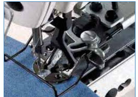
Oil-free, clean and durable machine thanks to the black diamond bar thread pick-up lever and the micro-oil lubrication system direct to the rotary hook. Fabrics are prevented from oil stains.
